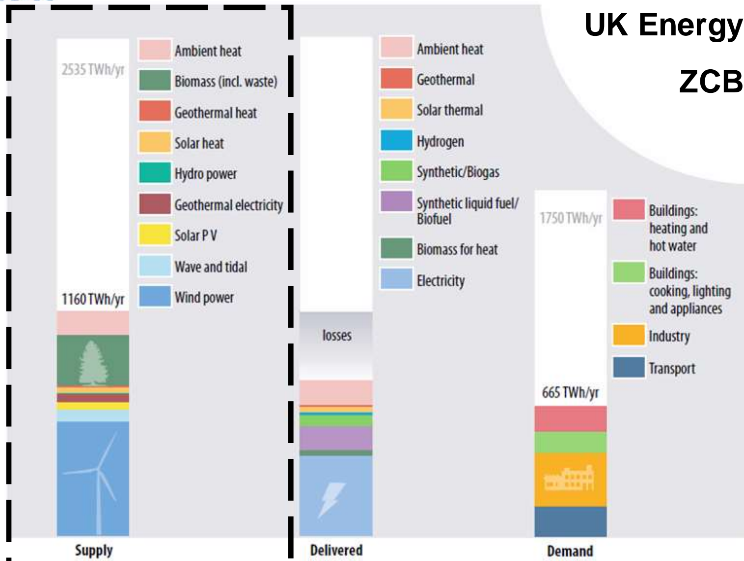
Figure 3.36: Primary energy supply, delivered fuel mix, and final energy demand for the UK in our scenario, relative to 2010.
